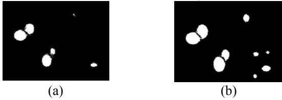
Fig. 2: Results obtained by the morphological flood-fill operation on Fig. 1(b): (a) without the application of CLAHE, (b) with the application of CLAHE.
