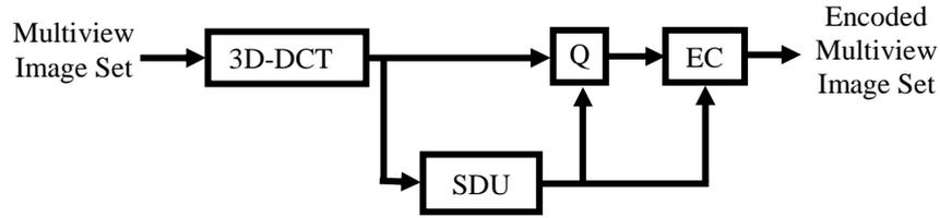
Fig. 4. Block diagram of an MDE encoder
