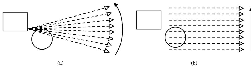
Fig. 1. Camera setup with (a) Convergent and (b) parallel axes.
