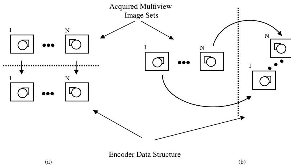
Fig. 2. Ordering of a multiview image set to form an image data volume (a) for the MDE and (b) for the 3D-DCT encoder
