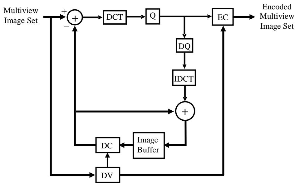
Fig. 3. Block diagram of an MDE encoder
