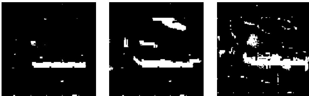
Fig. 5. Defect Detection results for the first textile image. From left to right the results obtained using the proposed feature extraction method, the 32 X 32 wavelet coefficients and the 32 X 32 pixel intensities as described in section 4.
