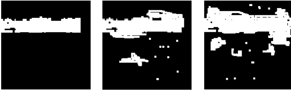
Fig. 6. Defect Detection results for the second textile image. From left to right the results obtained using the proposed feature extraction method, the 32 X 32 wavelet coefficients and the 32 X 32 pixel intensities as described in section 4.
