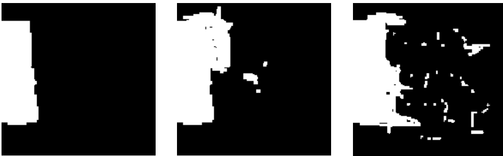
Fig. 7. Defect Detection results for the third textile image. From left to right the results obtained using the proposed feature extraction method, the 32 X 32 wavelet coefficients and the 32 X 32 pixel intensities as described in section 4.
